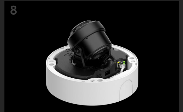
8 Power on (Connect the PoE cable)
